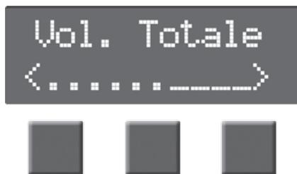
The parenthesis indicate that you are in selection mode; by pressing the side buttons you can scroll through the settings and, by clicking on the central button, you can modify them. When you confirm the settings to be modified, through the pressing of the central button, the parenthesis will disappear and the symbols + and - will appear.
