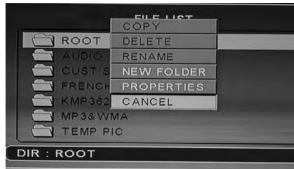
Press "UP / DOWN" direction keys to select operation, press "ENTER" key, then make the corresponding operation to the selected file.
